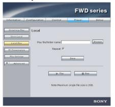
This screen lets you make settings for display and playback of still image and video files stored on a CF card inserted in the memory card slot of the BKM-FW50.
